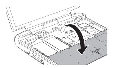
Figure 8-10 Removing the keyboard (3)
